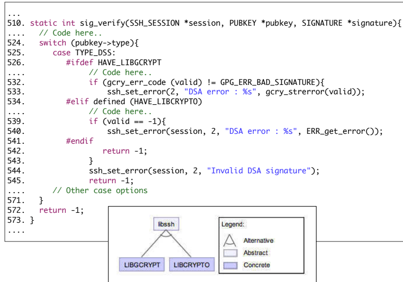
Figure 7.1: Code snippet of Libssh and its macro constraints.
