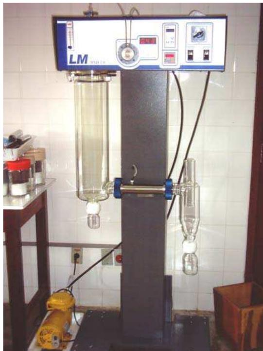
Figura 3.7 – Mini Spray Dryer Labmaq modelo MSD 1.0
