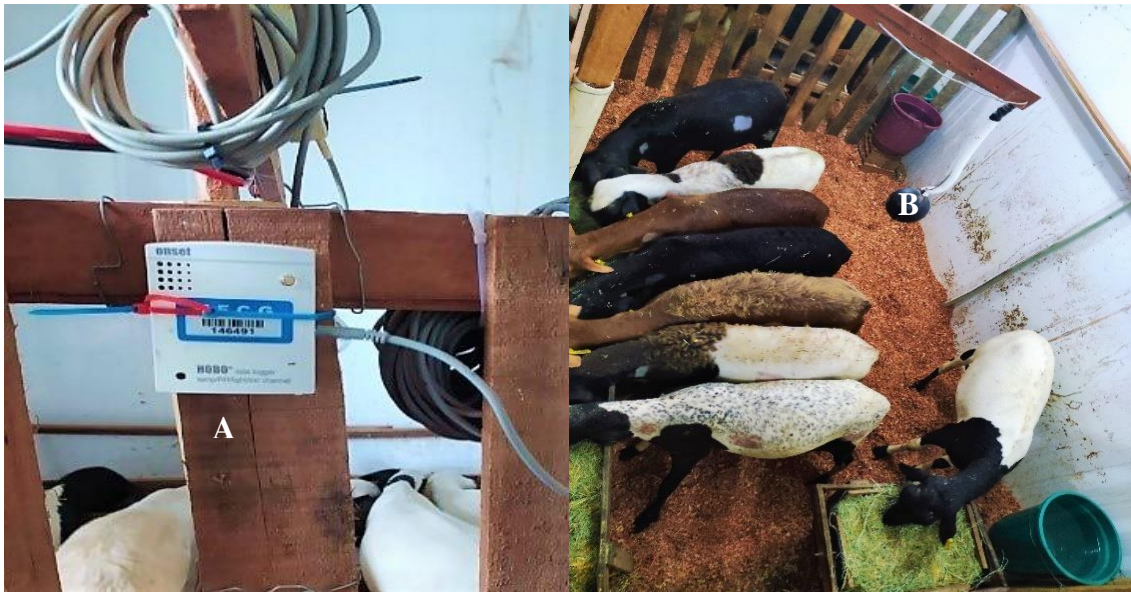
Figure 03: HOBOT-type datalogger (A), and external cable with the sensors attached to the black globe near the height of the animals in the central area of the stall (B). (Source: personal archive, 2021).
