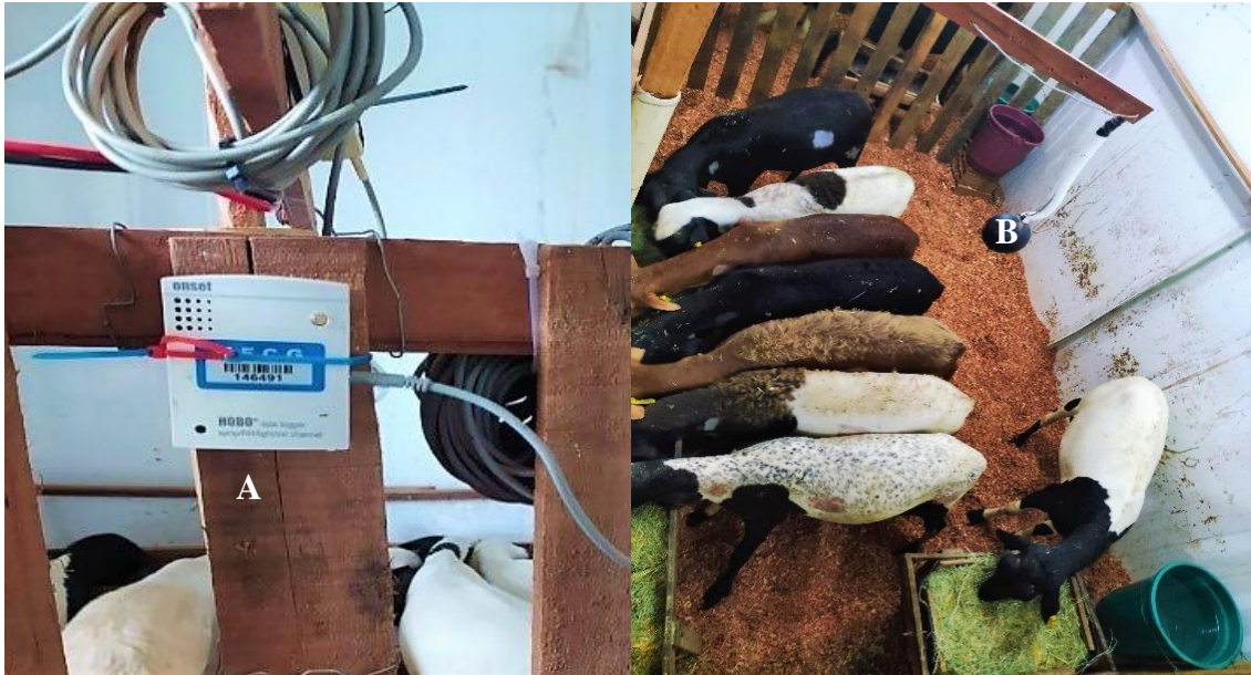
Figure 03: HOBO-type datalogger (A), and external cable with the sensors attached to the black globe, close to the height of the animals in the central area of the stall (B). (Source: personal archive, 2021).
