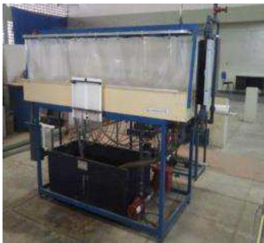
Figura 23 - Equipamento Basic Hydrology System (BHS)
