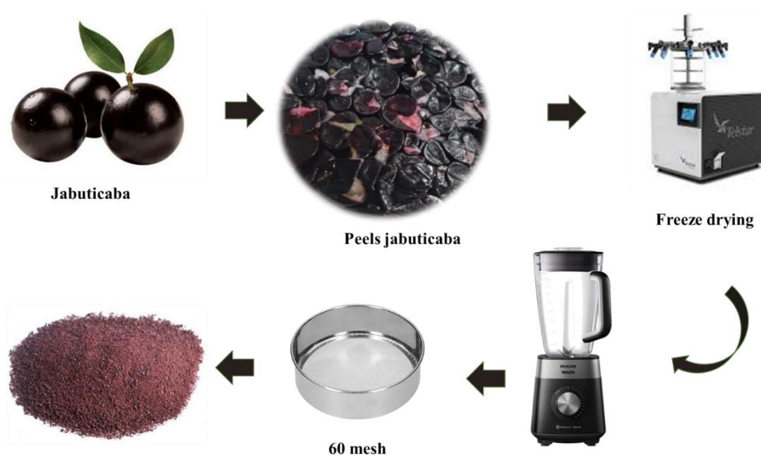
Figure 1. Main steps for the preparation of freeze-dried jabuticaba peel flour
