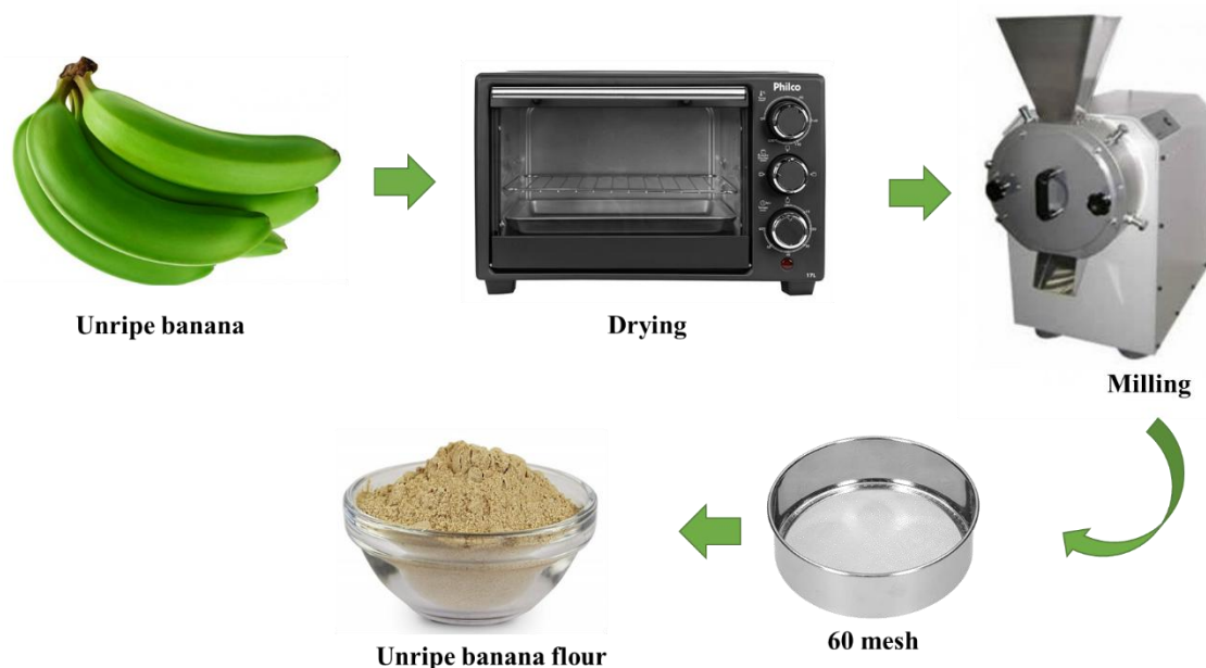
Figure 1. Main steps for the preparation of green banana peel flour.
