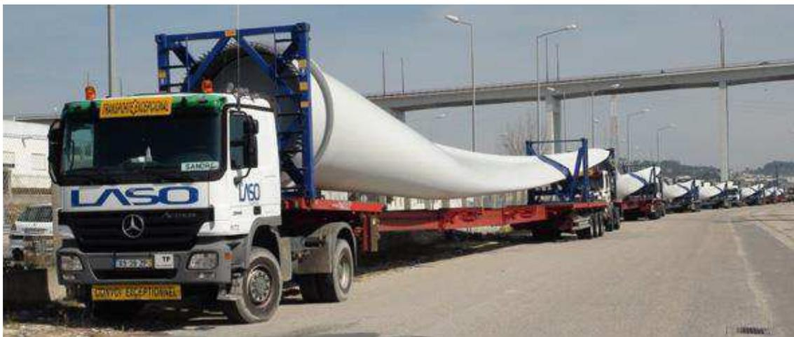
FIGURA 25 - PROCESSO DE TRANSPORTE DE PAS
