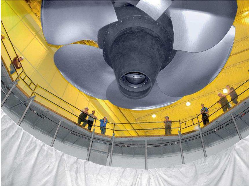
Figura 11: Turbina Kaplan.
