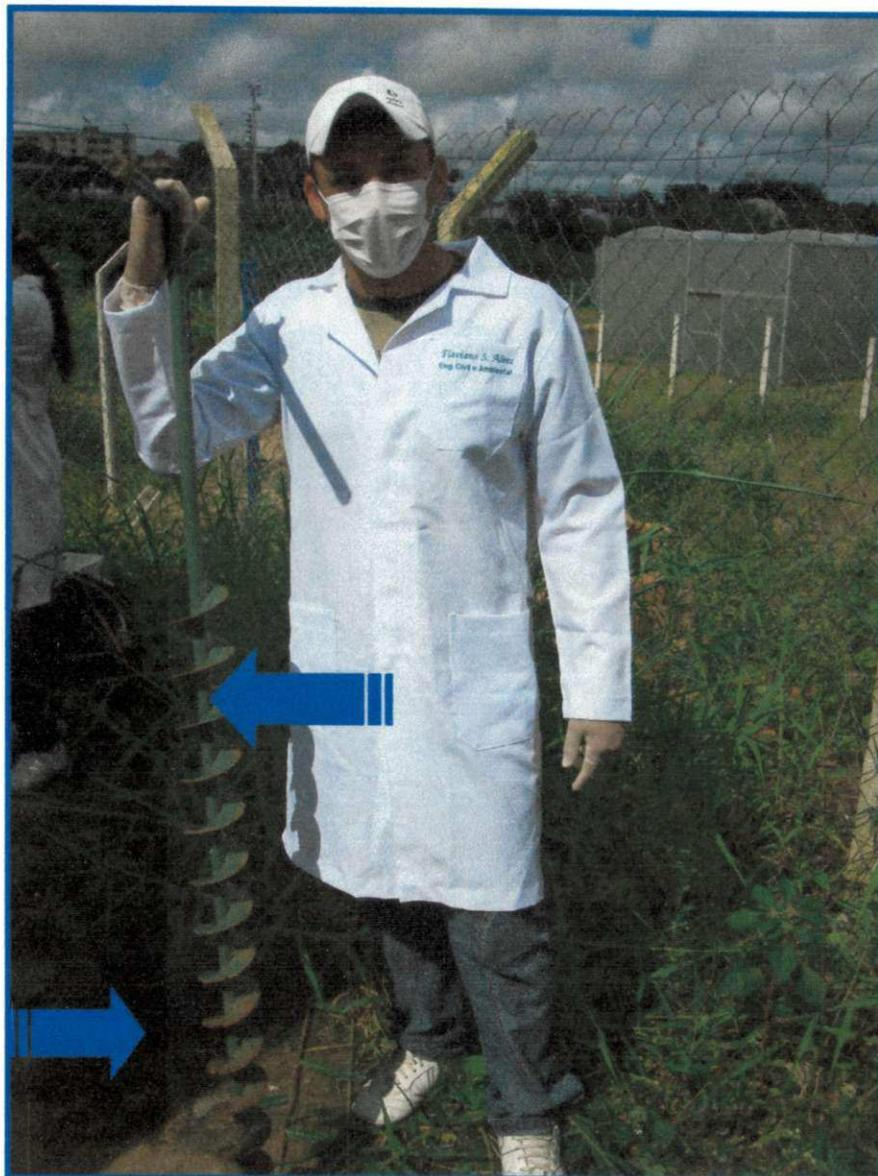
**Figura 45: Amostrador(Trado helicoidal) (GGA).**
