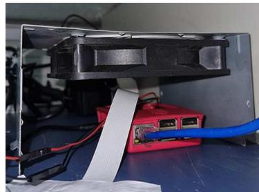
(b) Setup of the cooler and Raspberry.
