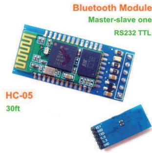
Figura 19 - Bluetooth RF Transceiver Module serial RS232 TTL HC-05.
