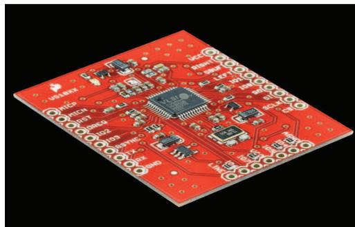
Figura 12 - MP3 and Midi Breakout Board for VS1053.
