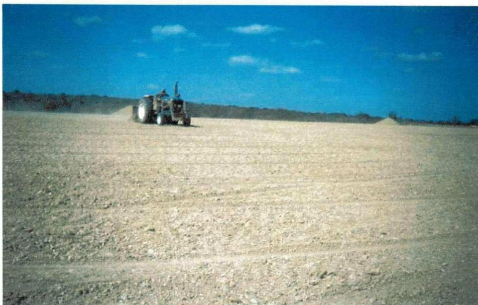
FIGURA 14 – SECAGEM NATURAL UTILIZANDO TRATORES PARA REMOVER AS ARGILAS ESTOCADAS.
